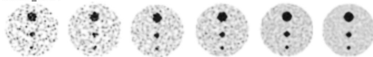
Fig. 11 Representative reconstructions obtained with MLEM-STOP (top) and MLEM-CONV (bottom). From left to right 10,000, 20,000, 35,000, 75,000, 150,000, and 300,000 counts simulated. For
