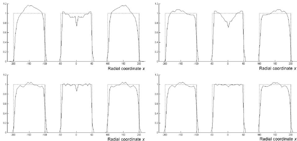
Fig. 7. Radial line profiles ( $y=0$  mm,  $z=61.6$  mm) through the object reconstructed from noiseless data. The dashed curves correspond to the exact line profile through the object. The completion was achieved using: *Top left:* reverse FORE. *Top right:* extended FORE. *Bottom left:* FOREPROJ. *Bottom right:* iterative FOREPROJ.
