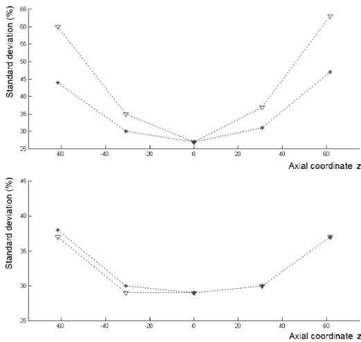
Fig. 9. Standard deviation calculated in the reconstructed ellipsoids (normalized to the mean pixel value in the ellipsoid) after completion using (triangles) reverse FORE and (stars) extended FORE. *Top*: ellipsoids situated on the scanner axis ( $x=0$  mm,  $y=0$  mm). *Bottom*: ellipsoids situated off-axis ( $x=150$  mm,  $y=150$  mm).
