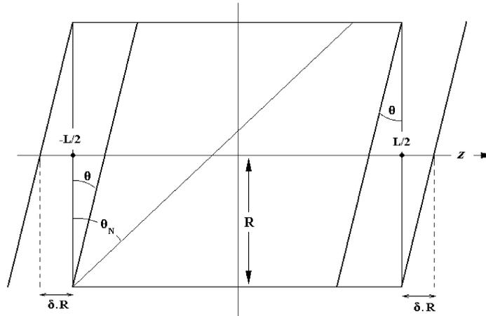
Fig. 2. The problem of the missing projections in the set of measured data: only segment 0 ( $\delta = \tan \theta = 0$ ) is axially invariant. Here,  $\theta_N = \text{atan}(\delta_N)$  is the aperture of the scanner, with  $\delta_N$  the maximum ring difference.
