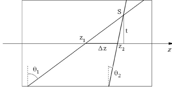
Fig. 3. Geometrical interpretation with the frequency-distance principle. S is a virtual source that contributes to the couple  $(\omega, k)$  in both sinograms  $(z_1, \delta_1)$  and  $(z_2, \delta_2)$ .
