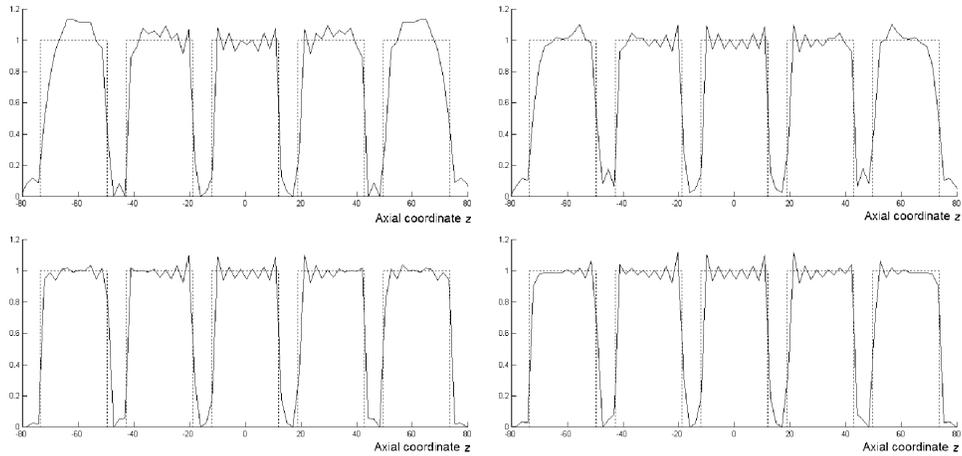
Fig. 8. Axial line profiles ( $x=0$  mm,  $y=150$  mm) through the object reconstructed from noiseless data. The dashed curves correspond to the exact line profile through the object. The completion was achieved using: *Top left*: reverse FORE. *Top right*: extended FORE. *Bottom left*: FOREPROJ. *Bottom right*: iterative FOREPROJ.
