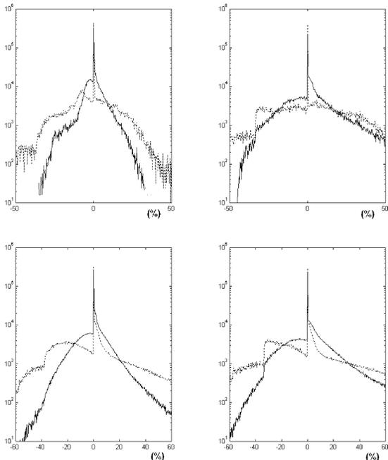
Fig. 5. Histogram of the difference (normalized to the data maximum) between the exact sinograms and the sinograms estimated from (top) noiseless and (bottom) noisy data. Comparison between reverse FORE (dashed) and extended FORE (solid). *Left*: Ring difference:  $\delta_3$ . *Right*: Ring difference:  $\delta_{10}$ .
