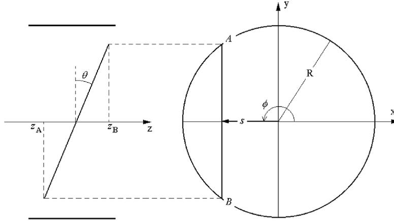
Fig. 1. Geometry of a PET scanner. *Left*: longitudinal section showing the axial variables  $z$  and  $\theta$ . *Right*: transaxial view. The standard sinogram variables  $s$  and  $\phi$  parameterize the straight line  $AB$ .
