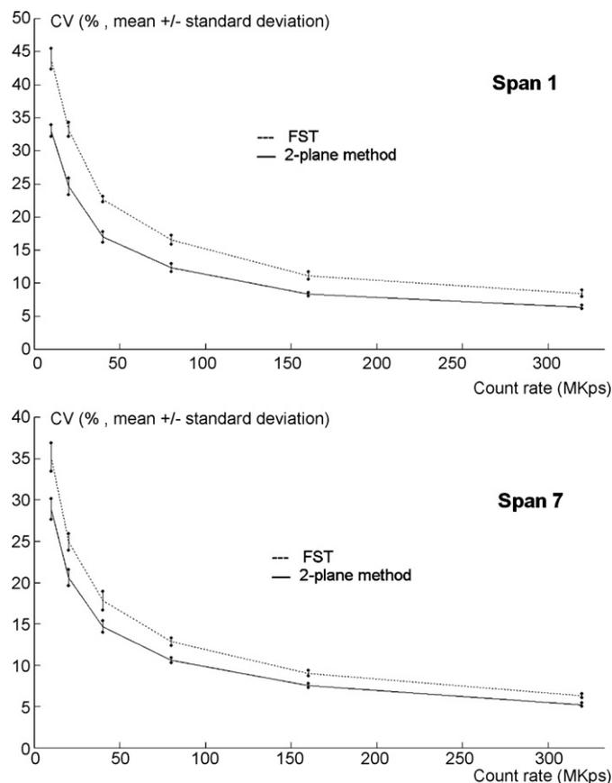
Fig. 7. Evolution with the counting rate of the mean CV ( $\pm$ S.D.) calculated in the axial range where the shift-invariance is achieved ( $|x_3| < 9$  mm for span 1,  $|x_3| < 21$  mm for span 7).
