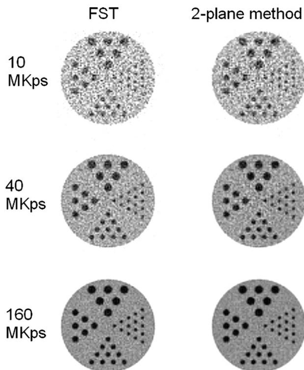
Fig. 8. Reconstructions of a Derenzo-like phantom with 10, 40 and 160 million simulated events. The figure shows the results achieved with the two algorithms tested.
