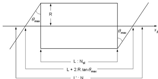
Fig. 2. Explanatory diagram for the computation of the axial sampling  $N_{ax}$ .
