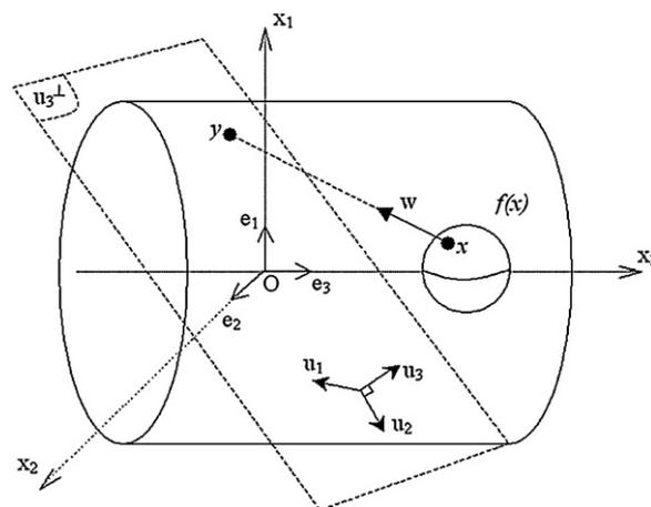
Fig. 1. Illustration of the projection of an unknown 3D radioactive distribution  $f(x)$  onto a projection plane  $u_3^\perp$ .
