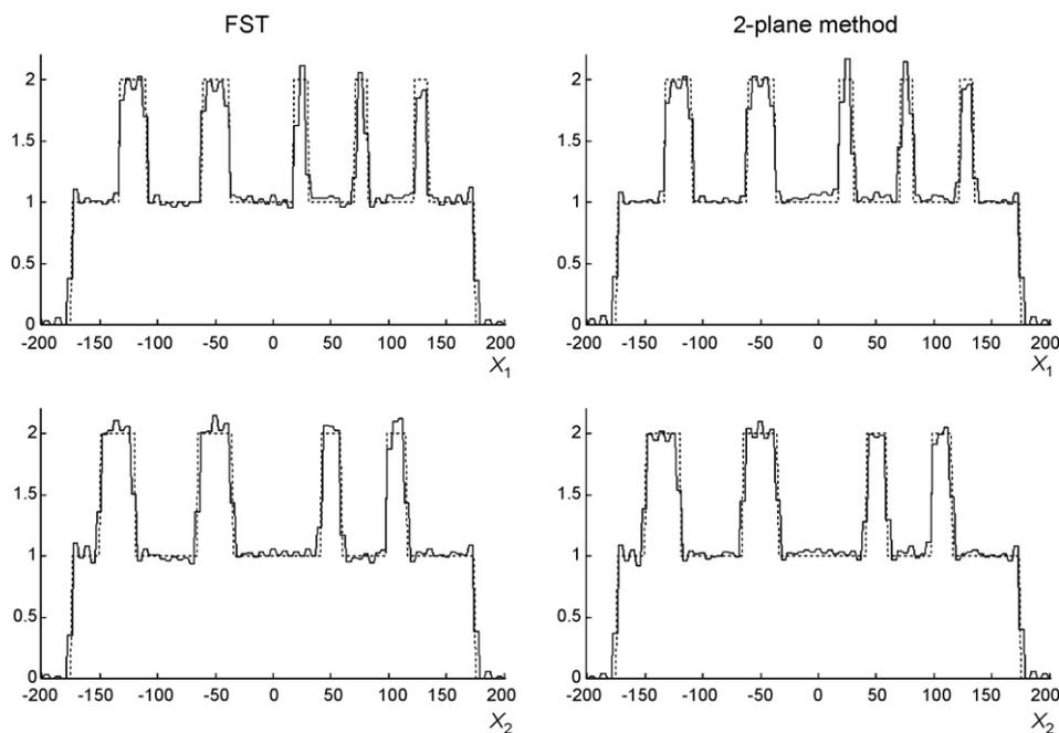
Fig. 5. Central line profiles along the two transverse axes through the reconstructions of a Derenzo-like phantom simulated with a span equal to 7 and without noise.
