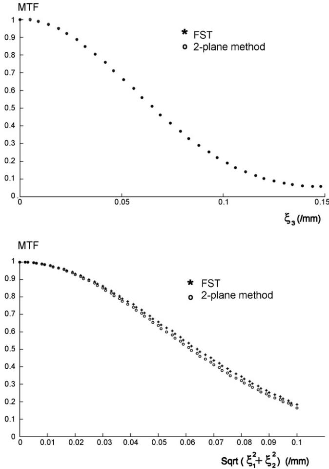
Fig. 4. Transaxial (top) and axial (bottom) modulation transfer functions (MTF) at the center of the field of view for the usual implementation of the Fourier slice theorem and for the two-plane method.  $\sqrt{\xi_1^2 + \xi_2^2}$  and  $\xi_3$  are the transaxial and axial spatial frequencies.
