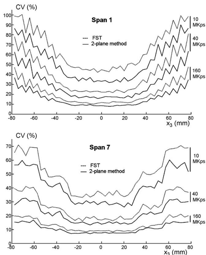
Fig. 6. CV in the transaxial slices measured for the two algorithms in a cylindrical phantom with a span set to 7 (bottom) or 1 (top). Three counting rates are evaluated: 10, 40 and 160 MKps.
