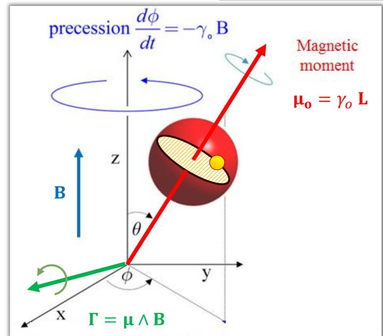
$\frac{d\mathbf{L}}{dt} = \boldsymbol{\mu}_o \wedge \mathbf{B}$        $\frac{d\boldsymbol{\mu}_o}{dt} = \gamma_o \boldsymbol{\mu}_o \wedge \mathbf{B}$
