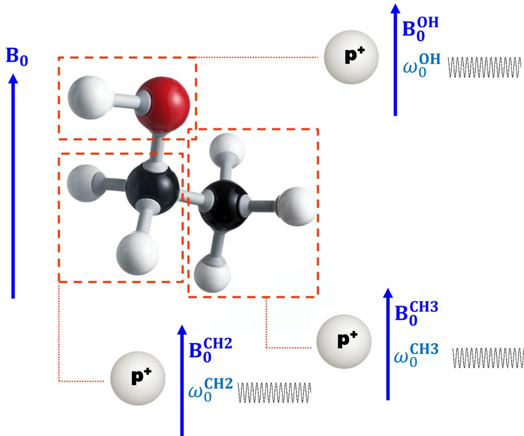
FID = signal (OH) + signal(CH<sub>2</sub>) + signal(CH<sub>3</sub>)
