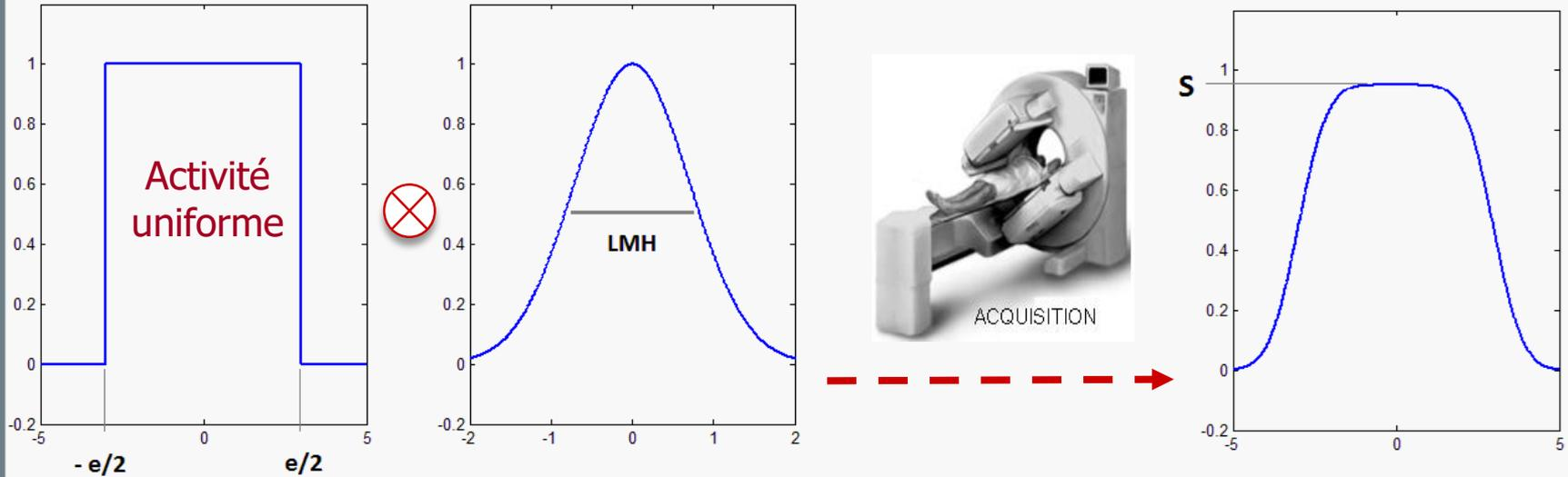
$$S = \int_{-e/2}^{e/2} G(x) dx = \frac{2\sqrt{\ln 2 / \pi}}{LMH} \int_{-e/2}^{e/2} e^{-\frac{4 \ln 2}{LMH^2} x^2} dx$$
