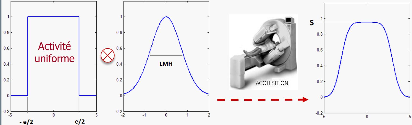
$$S = \int_{-e/2}^{e/2} G(x) dx = \frac{1}{\sigma\sqrt{2\pi}} \int_{-e/2}^{e/2} e^{-\frac{x^2}{2\sigma^2}} dx$$
